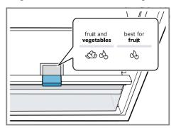
The air humidity in the fruit and vegetable container can be set according to the type and amount of food to be stored by pressing the humidity controller:
