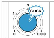
The temperature controller (refrigerator compartment) locks into place for the duration of the defrostina process.
