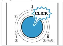
The temperature controller (refrigerator compartment) locks into place for the duration of the defrosting process.
