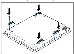
**4.** Turn the cooktop around and insert it into the recess. Insert the cooktop in the front of the recess.
