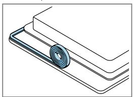
3. Screw the brackets supplied into the specified position so that they can turn freely.
