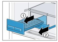
2. Lift the fixed shelf with the holder at the rear 1 and remove it 2.
