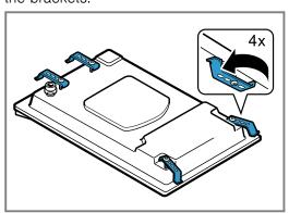
3. Turn the hob around and insert it into the recess. Insert the hob in the front of the recess.
