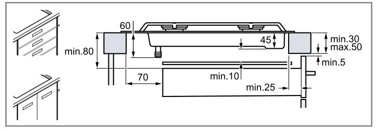
To avoid leaking gas to accumulate and cause an explosion, ensure that the cabinet on which the built-in cooking appliance is mounted has an air outlet to the surrounding room with a minimum crosssection of 100 cm<sup>2</sup>.
