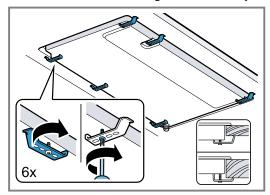
The position of the brackets depends on the worktop thickness.
