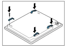
**4.** If you install the appliance in a 480 mm wide niche, you must remove the spacer, which is preinstalled on the back of some models.
