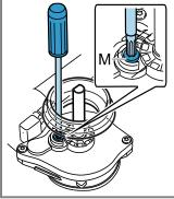
Never remove the sealing ring. The sealing rings prevent liquids and dirt from finding their way into the appliance and impairing its ability to function properly.
