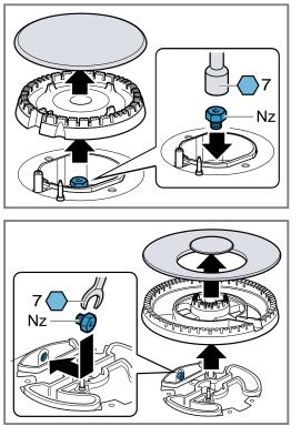
Ensure that the nozzle does not become detached during removal or fastening.
