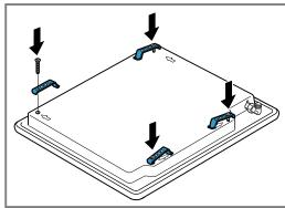
**4.** If you install the appliance in a 480 mm wide niche, you must remove the spacer, which is preinstalled on the back of some models.
