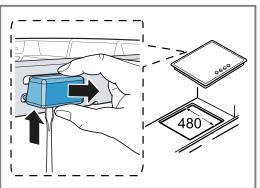
5. Turn the cooktop around and insert it into the recess. Insert the cooktop in the front of the recess.
