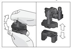
■ Separate the milk tubes, connecting element and suction pipe.
