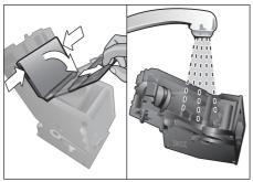
■ Clean the strainer of the brewing unit thoroughly under the water jet.
