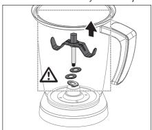
**4.** Hold the blade assembly with cloth. Using spatula untighten the blade nut (turn in a clockwise direction).
