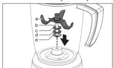
Put 2 x fibre- and metal washer onto the axis from the underside and tighten the coupler by rotating it in an anti-clockwise direction.
