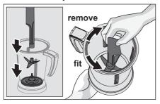
**Note:** If the coupler and/or some other parts are removed during removing the blade, please refer to → "Blade changing procedure" see page 9.
