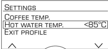
The different setting options can be selected with the selection buttons **^** and **v**.
