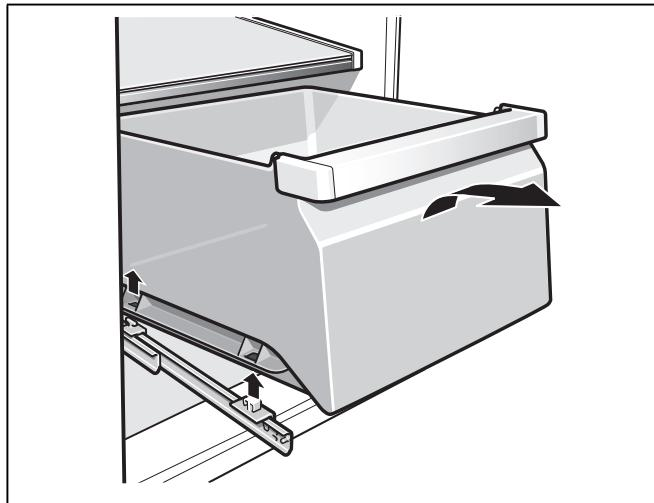
To insert the container, place on the telescopic rails and push into the appliance. Attach the container by pressing it down.
