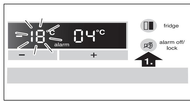
The temperature display indicates for 10 seconds the warmest temperature which was reached in the freezer compartment. Then the set temperature is displayed again.
