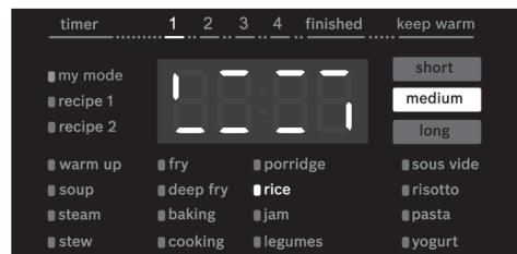
The appliance heats up the pan until the target temperature is reached. During the heating phase, lines that light up in a clockwise direction appear in the display. Once the target temperature is reached, the lines go out and the preparation time is shown in the display.
