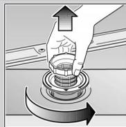
Rotate filter cylinder, remove filter system
