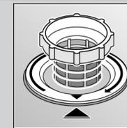
Screw on filter system. NOTE MARK!
