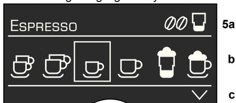
The status line **5a** in the display **5** shows the name of the type of drink, along with the strength setting, e.g. **00** and per-cup quantity, e.g. **1**. The selection line **5b** shows symbols for drink selection.
