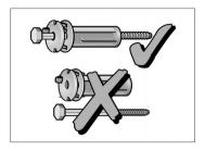
Always keep the transport bolts for subsequent transportation of the appliance (e.g. when moving house).
