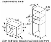
Bean and water containers are removed fro the front Recommended installation height 950–1450 mm
