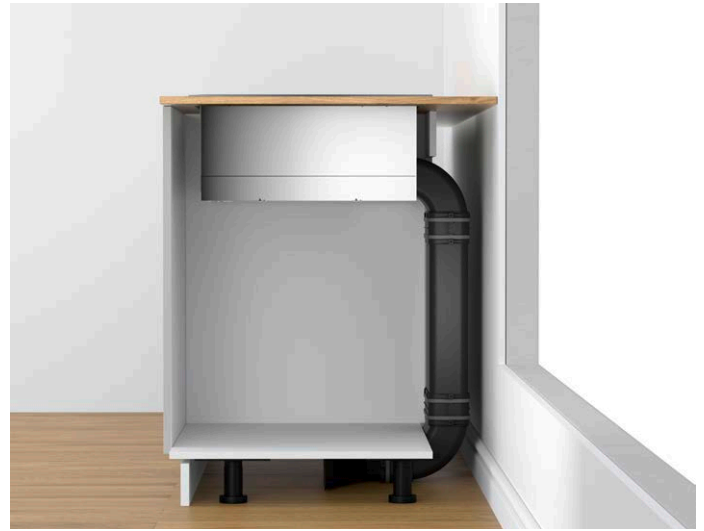
Next to uninsulated exterior walls ( \mu \geq 0,5 \text{ W/m}^2 \text{ }^\circ\text{C} ), a partly or fully ducted recirculation configuration is recommended in order to minimize any potential condensation risk.
