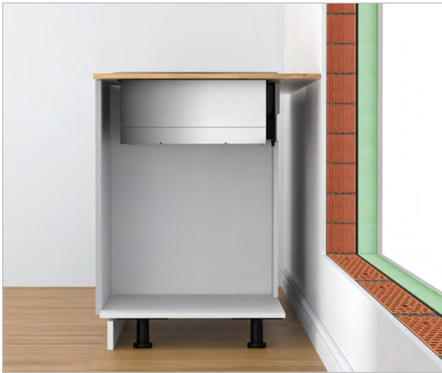
Next to well-insulated exterior walls ( \mu < 0,5 \text{ W/m}^2 \text{ }^\circ\text{C} ), all recirculation configurations are possible.
