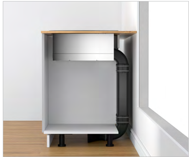
Next to uninsulated exterior walls ( \mu \geq 0,5 \text{ W/m}^2 \text{ }^\circ\text{C} ), a partly or fully ducted recirculation configuration is recommended in order to minimize any potential condensation risk.
