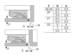
The gap dimensions recommended in the table must be adhered to in order to ensure that appliance doors do not collide with anything when they are opened, and to avoid causing damage to kitchen units.
