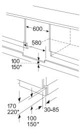
Space for electrical connection next to the appliance on the left or right-hand side. Ventilation space in the base.
