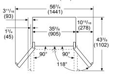
Drawers can be pulled out with door open to  $90^{\circ}$ Drawers can be taken out with door completely opened
