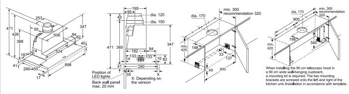
DFR097A50A measurements in mm
