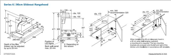
measurements in mm
