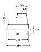
DHL555BAU measurements in mm
