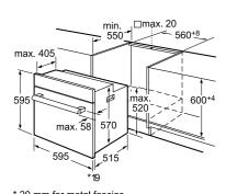
\* 20 mm for metal fascias Measurements in mm
