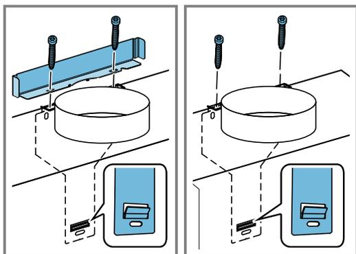
When you install a flue cover, install the bracket and hold it in place while screwing it in tight.
