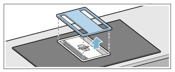
2. Remove the metal grease filter and container.
