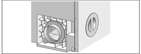
The exhaust air opening on the back panel is open when the dryer is delivered (bayonet ring). The exhaust air opening on the left side panel is sealed with a cover.
