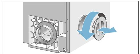
2. Remove the bayonet ring from the back panel and attach it to the opening on the side panel.
