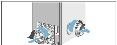
3. Seal the opening in the back panel with the cover.
