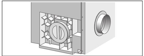
You can switch the connection on the back panel to the left side panel as follows:
