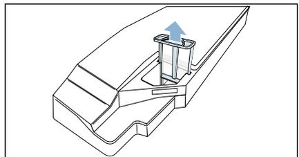
11. Place the filter into the recess on the condensation container.
