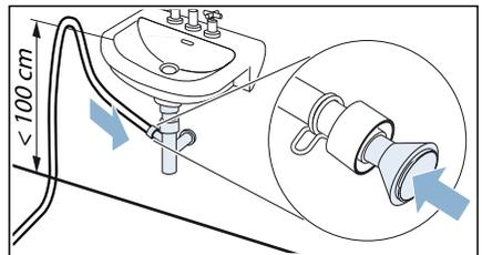
The connection point must be secured using a hose clamp (clamping range 12-22 mm).
