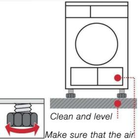
Clean and level. Make sure that the air inlet remains unobstructed.
