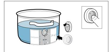
**3.** Press down all over the surface of the silicone patch, including in the centre.
