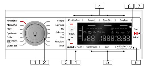
**Note:** All the buttons are sensitive (except for the main switch) and only need to be pressed lightly.
