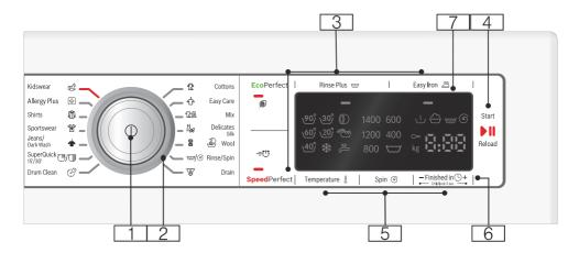
**Note:** All the buttons are sensitive (except for the main switch) and only need to be pressed lightly.
