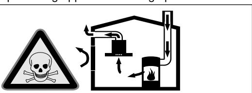
Room air-dependent heat-producing appliances (e.g. gas, oil, wood or coal-operated heaters, continuous flow heaters or water heaters) obtain combustion air from the room in which they are installed and discharge the exhaust gases into the open air through an exhaust gas system (e.g. a chimney).
