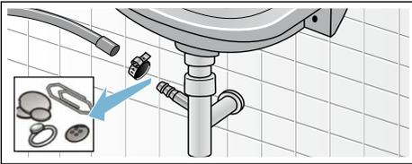
4. Re-attach the drain hose and secure the connection point using the hose clamp.
