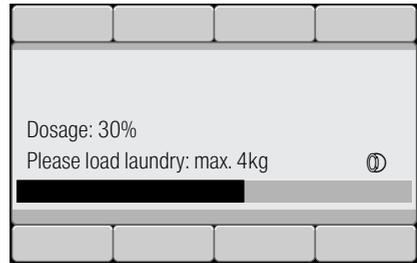
The load bar fills as the laundry is loaded. If the maximum load is exceeded, the bar flashes. Observe the maximum indicated load. Overfilling adversely affects the washing result and encourages creasing.
