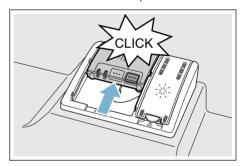
The detergent dispenser opens automatically at the optimum time depending on the programme. The powder or liquid detergent is distributed in the appliance and is dissolved, the tablet falls into the tablet collecting tray where it dissolves in doses.
