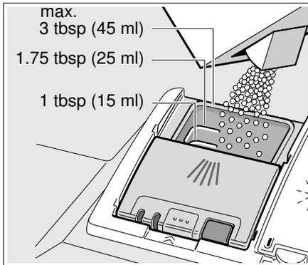
When using detergent tabs, lay them such that they do not come in contact with the cover, insert a detergent tab flat, not on its side.
