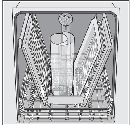
**Note:** Keep the vent hole [25] on the tub's left side clear by placing tall items such as plastic cutting boards and tall baking sheets on the lower rack's right side or center.
