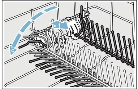
Upper rack flip tines: To fold down, push flip tines downward with gentle pressure. To fold up, push flip tines into an upright position until the holder engages in the notch.
