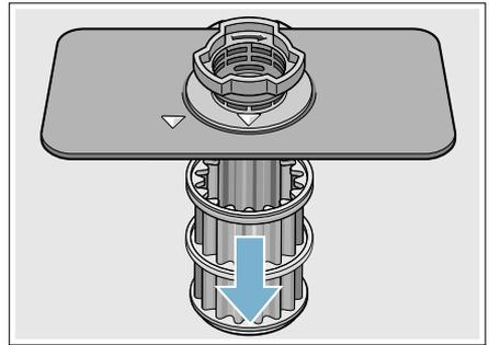
2. Remove any residue and clean filters by rinsing under running water. Note: do not use abrasive brushes or steel wool, etc., as they may damage the filter.
