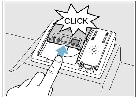
The detergent dispenser will open automatically at the ideal time for the set cycle. The powder or liquid detergent is distributed in the appliance and is dissolved, detergent tabs will fall into the detergent tab tray [24] where it dissolves during the cycle.
