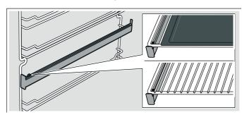
**Note:** The rotary spit must be inserted on level 1. In this case, move the pull-out rails for the baking tray and the baking and roasting shelf to the four upper levels.
