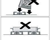
Never use two burners or heat sources to heat one single pan.
