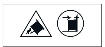
**Warning:** In order to prevent tipping of the appliance, this stabilizing means must be installed. Refer to the instructions for installation.
