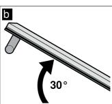
4. Raise the oven door slightly and pull it out. Note: Do not fully close the oven door. The hinges could become bent and the enamel could be damaged.
