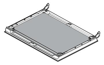
**Note:** The two middle panels are not fastened using retaining pins; instead, they are held in place using holders.
