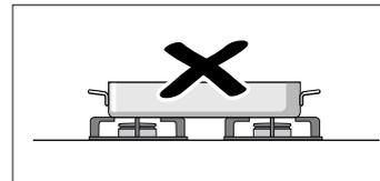
Never use two burners or heat sources to heat one single pan.
