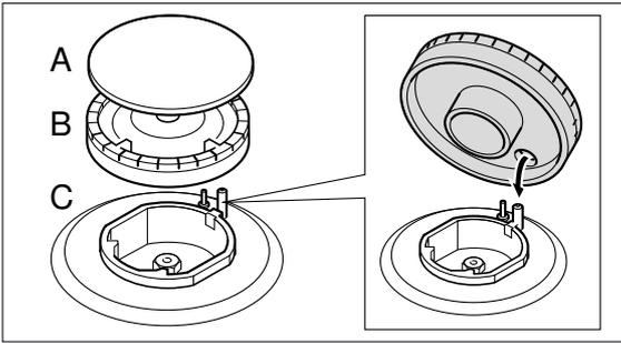
1. Clean the burner caps (A) and cups (B) with water and washing-up liquid.
