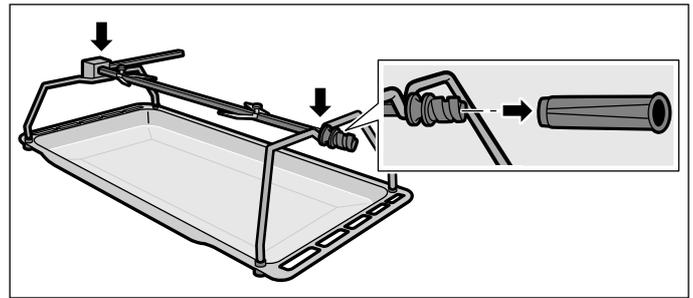
3. Slide the universal pan into shelf position 1 and slide the rotary spit into the motor mount.
