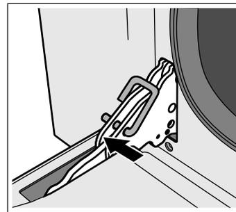
3. Lift the bottom of the inner panel slightly until the fastening pins come out of the holder (1).
