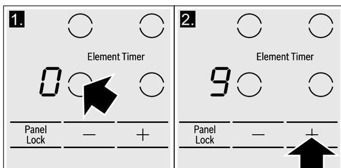
3. To change the power level, touch the **+** or **-** key until the desired power level is displayed.
