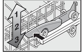
The RackMatic® can be adjusted to 9 different positions and heights on opposite sides to create **Ter-raced Racks** (see RackMatic® description on page 5) for increased flexibility.
