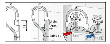
Attach the drain hose to the elbow included with your washer.
