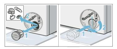
Turn the pump cover counterclockwise to remove it. A small amount of residual water may flow out when the cover is removed.
