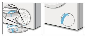
**8.** Snap the service cover in place at the hinges and close it. Wipe up any spilled water.
