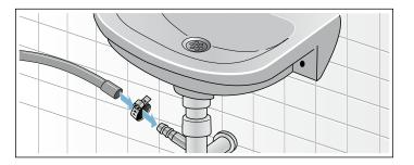
Secure the drain hose to the sink siphon using a  $\emptyset$  0.9 - 1.6 in. (20-44 mm) hose clip (available from a hardware store).
