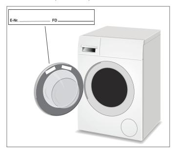
The **E-Nr.** (model number) and the **FD** (serial) number are found on the rating plate label.
