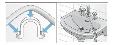
Attach the drain hose securely to the wash basin.
