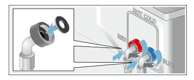
Attach this end of the hose to the back of the washing machine as shown in the following pictures. Be sure to use clamps and route hoses as instructed. Hand tighten only.
