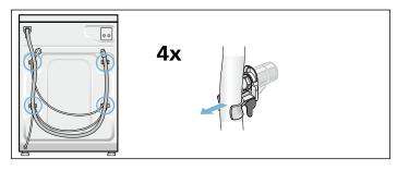
Loosen and remove all 4 transport bolts. Remove the sleeves. Take the power cable out of the brackets.
