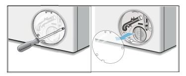
**4.** Loosen the screws and remove the protective film.
