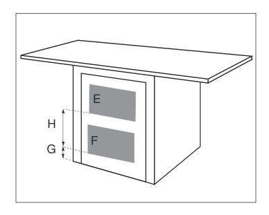
If front of the appliance is covered ventilation openings must be installed.
