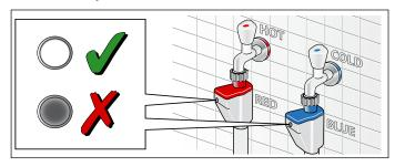
The AquaShield® hose prevents potential flooding in the event the hose develops an internal leak. If the hose leaks, the indicator turns red and water flow is blocked. Once the internal valve in the hose activates (indicator is red) the hose must be discarded. Contact customer service for a replacement.
