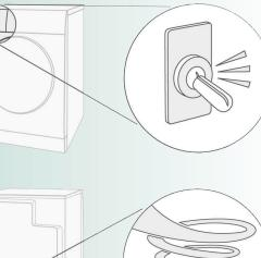
The process of pumping the condensation into the condensation container generates pumping noises.
