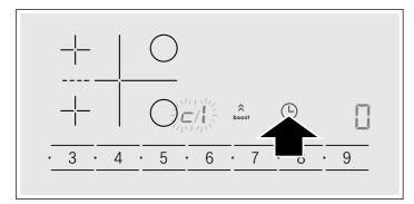
${\it c}$  and  ${\it I}$  flash alternately in the heat setting display and  ${\it I}$  appears in the timer display as a preset.
