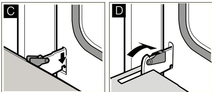
The appliance door is secured and can no longer be removed.
