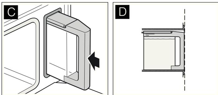
The tank must be flush with the water tank recess (fig. D).
