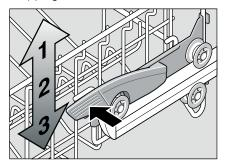
To raise the basket, hold the basket on the sides of the upper edge and lift it up.  Before re-inserting the basket again, ensure that it is at the same height on both sides. Otherwise, the appliance door cannot be closed and the upper spray arm will not be connected to the water circuit.
