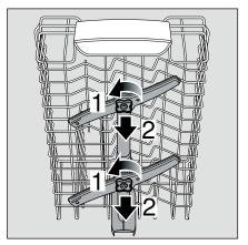
Remove the lower spray arm 24 upwards.
