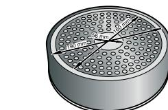
For good cooking results, the diameter of the cookware's ferromagnetic area should match the size of the hotplate. If cookware is not detected on a hotplate, try it on the next smaller hotplate down.
