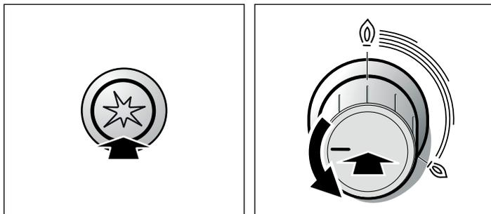
4. Press and hold the burner knob for approximately 1-3 seconds. The safety pilot is activated. If the gas flame goes out, the gas supply is automatically interrupted by the safety pilot.
