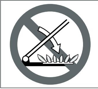
**Caution:** The glass cover may crack due to heat. Before closing the cover, turn off all burners. Wait until the oven has cooled down before closing the glass cover.
