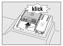
The detergent dispenser opens automatically at the optimum time depending on the programme. The powder or liquid detergent is distributed in the appliance and is dissolved. The tablet falls into the appliance and dissolves.
