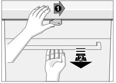
To open the door, move lever to right and pull door handle.
