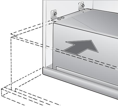
**Important:** The extractor hood must be firmly seated on the 4 mounting brackets.
