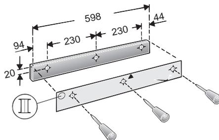
2. Align handle and attach it to the extractor with the 3 enclosed screws.
