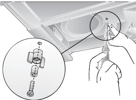
– Screw, sleeve and wing nut are enclosed with the activated carbon filter –.
