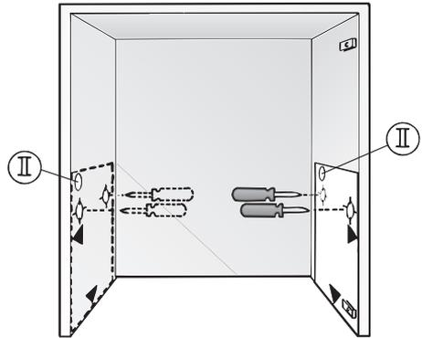
3. Align the 4 enclosed mounting brackets and screw them on tight.
