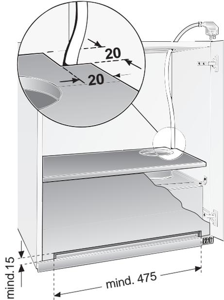
⚠ If the shelf is permanently fixed inside the cupboard, 4 holes must be drilled to provide access to the 4 mounting screws for the extractor hood.
