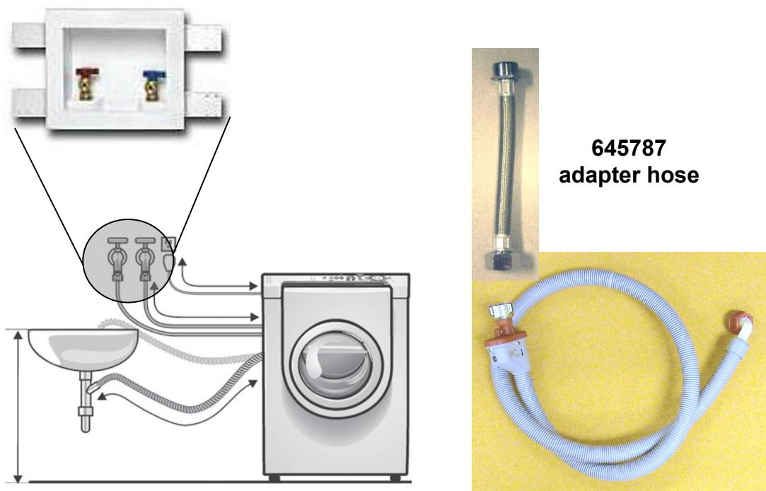
For many installations, (2) **645787** adapter hoses will be needed – (1) for the hot water hose and (1) for the cold water hose.
